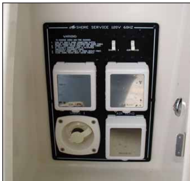
120-Volt Inlets and Breakers
