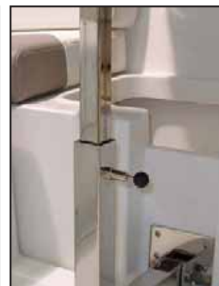
Spring Loaded Lock Pin on Table Pedestal
