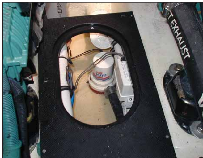
Automatic Float Switch for High Water Alarm and Emergency Bilge Pump Located Below the Engine Compartment Floor.
