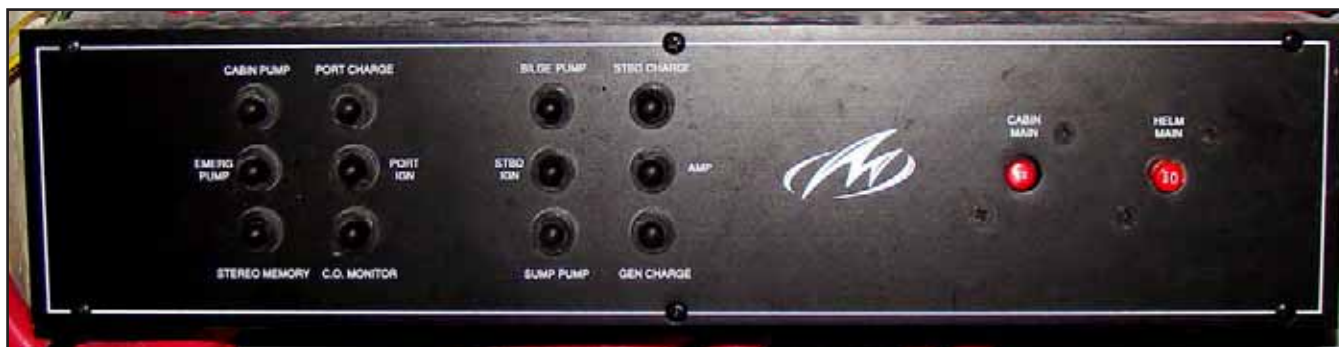
Constant Hot and Switched Circuit Breaker Panel Near Battery Switches in Engine Compartment
