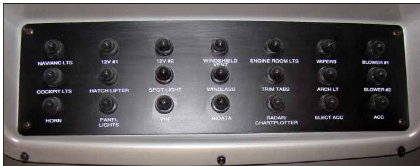
Helm Circuit Breaker Panel Located in the Helm Station Below the Steering Wheel
