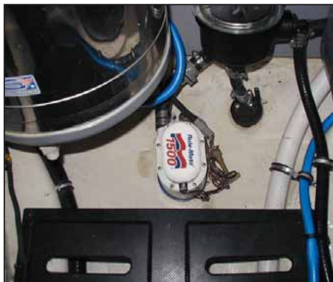
Aft Bilge Pump and Automatic Float Switch
