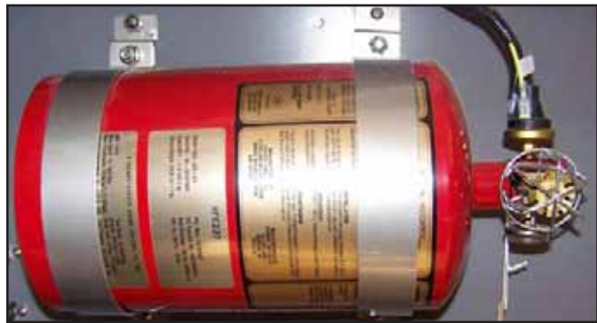
Typical Automatic Fire Extinguishing System in the Engine Compartment
