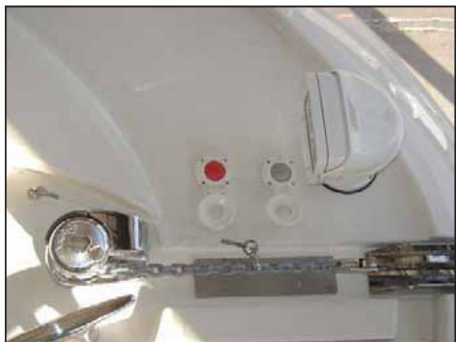
Windlass, Chain Binder, Windlass Deck Switches and Optional Spot Light
