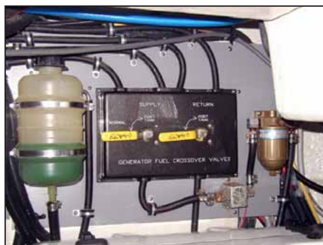
Typical Diesel Generator Coolant Recovery Tank, Fuel Crossover Valves, Fuel Supply Pump and Fuel Filter
