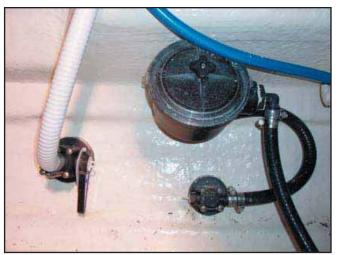
Holding Tank Overboard Discharge Thru-Hull Valve
