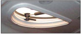
Galley Deck Hatch Secured in Vent Position
