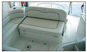
Cockpit Lounge Seat in the Aft Position (the backrest should be in this position whenever the engines are running)
