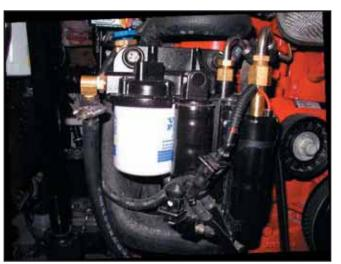
Typical Gas Engine Fuel Filter
