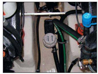
Aft Bilge Pump and Automatic Float Switch
