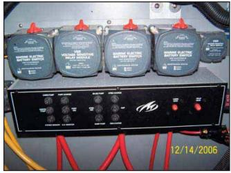
Battery Selector Switches, Circuit Breakers and Charging Relay
