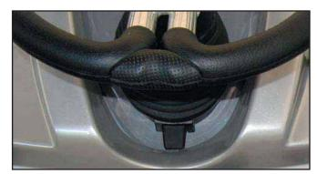
Steering Wheel Tilt Adjustment Lever
