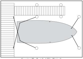
Securing The Boat In A Slip (Typical)
