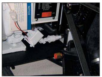
Typical Gasoline Generator Fuel Filter
