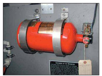
Automatic Fire Extinguishing System in the Engine Compartment
