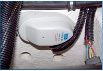
Air Dome Switch for High Water Alarm and SeaKey (Optional)
