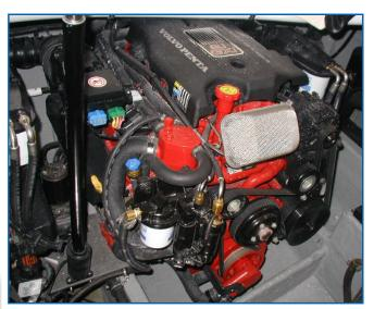
Volvo Gas Engine Equipped With Fresh water Cooling
