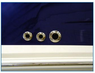
Cockpit Scupper Thru-Hull Fitting
