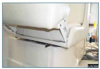
Helm Seat Bolster Up and Adjustment Lever
