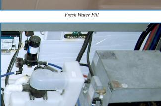
Fresh Water Pump, Water Heater and Waste System Vacuum Pump
