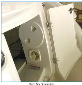
To use shore water, connect a hose from the shore water faucet to the shore water fitting located in the transom storage compartment. Next, turn on the shore water. The pressure pump will not run and the water in the boat's water tank will not be used.
