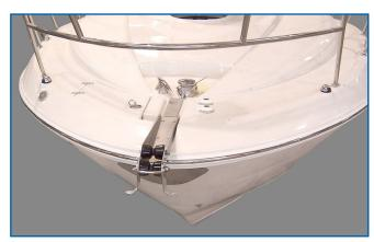
Roller Assembly and Rope Locker
