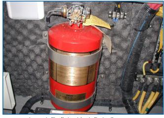
Automatic Fire Extinguisher in Engine Compartment
