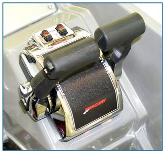
Mercruiser Engine Controls and Control Head
