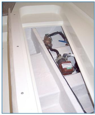
Air Conditioning, Thru-Hull Valve, Pump and Strainer
