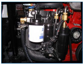
Typical Gas Engine Fuel Filter
