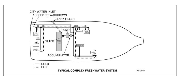
Pressurized systems can range from the simple type consisting of a storage tank, electric pump and faucet, to the complex type consisting of a storage tank, filter, electric pump, accumulator, city water hookup, water heater, and any one of a number of showers, sinks, or other items which require potable water.
