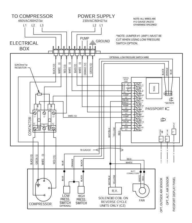
**VECTOR SERIES AIR CONDITIONER SELF CONTAINED UNIT WIRING DIAGRAM**
