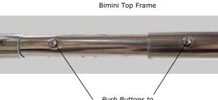
Push Buttons to adjust Canvas Frame. Ensure buttons are engaged before boat is in operation.
