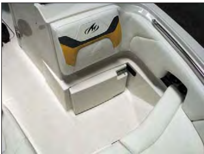
M3 with Bow Lounge Seat Cushion Removed and Foldout Support Latched in the Stored Position
