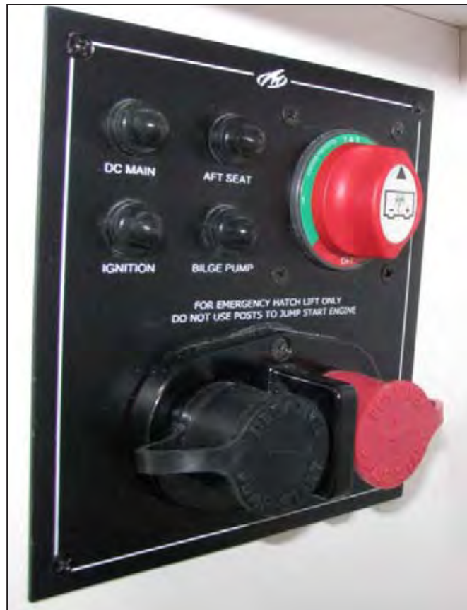
M5 Dual Battery Switch Panel with Circuit Breakers and Engine Hatch Jumper Terminals
