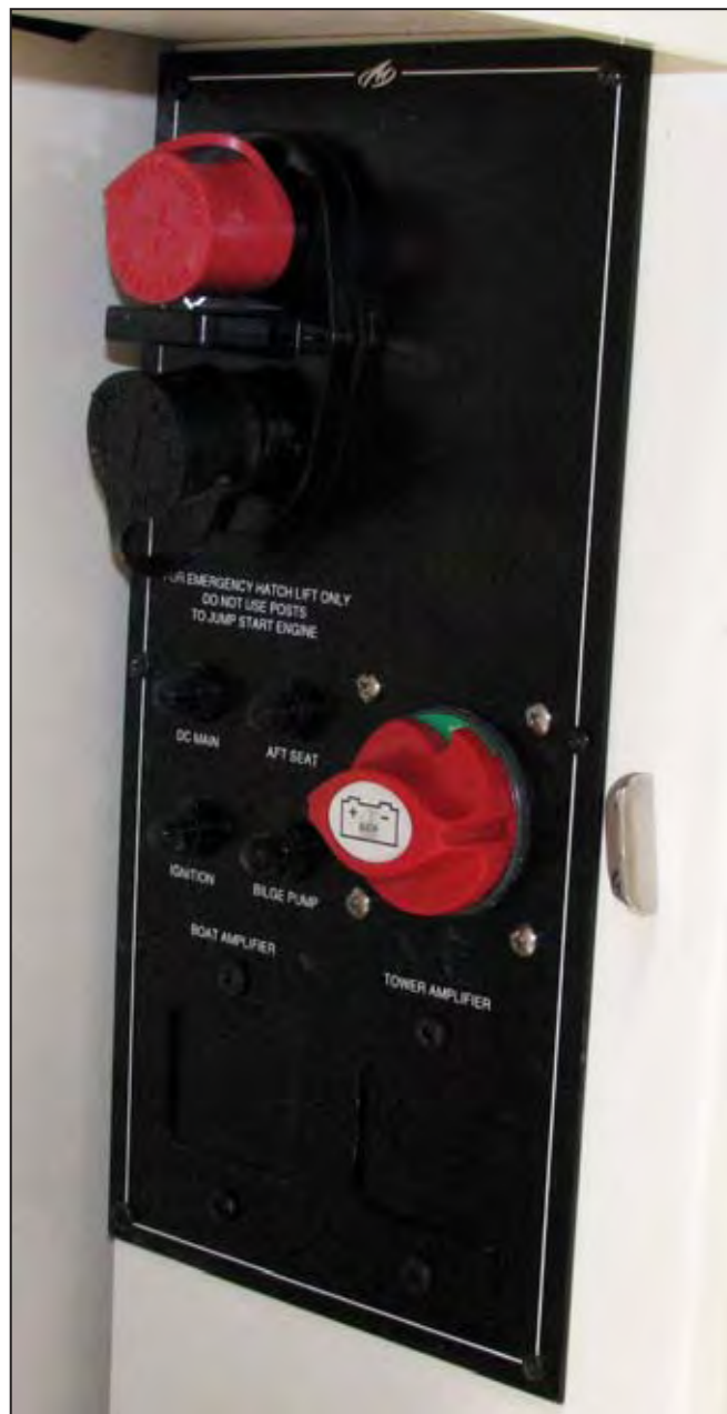
M3 Single Battery Switch Panel with Circuit Breakers and Engine Hatch Battery Jumper Terminals
