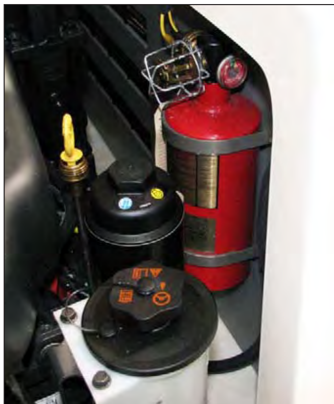
Automatic Fire Extinguishing System in the Engine Compartment
