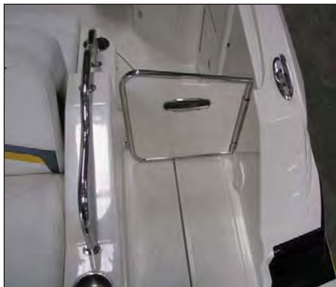
Transom Door Closed (Door must be in the open position to open the engine hatch)
