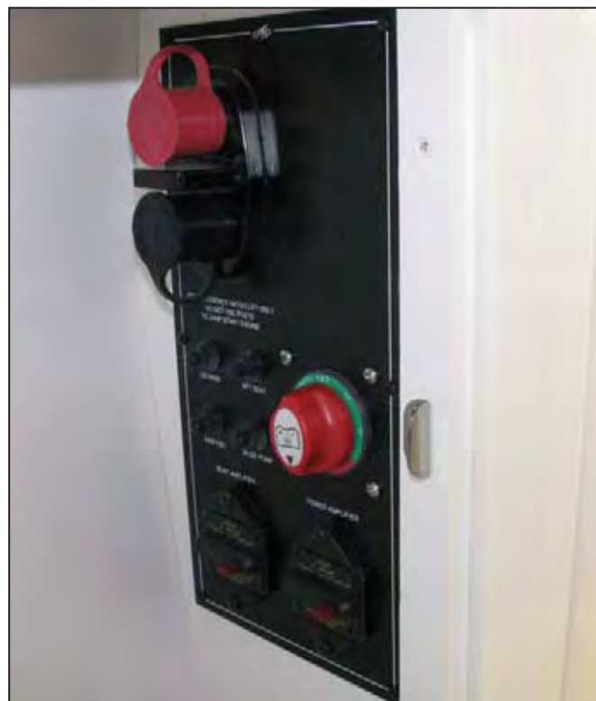
MSX Dual Battery Switch Panel w/ Circuit Breakers, Engine Hatch Jumper Terminals and Sound System Amplifiers
