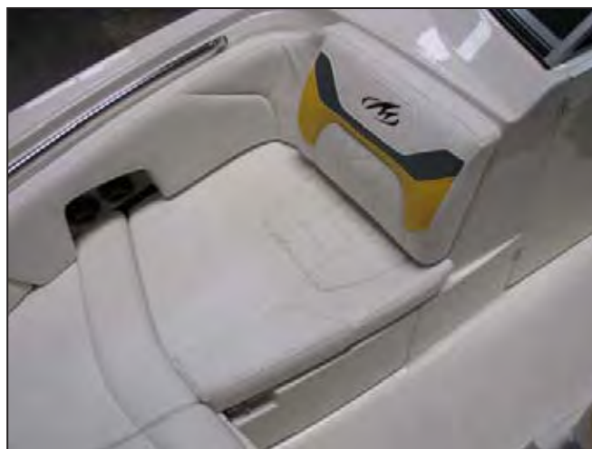
M3 with Bow Lounge Seat Cushion Installed and Foldout Support Latched in the Open, Seat Support Position
