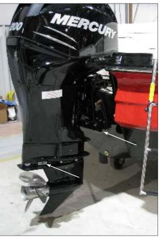
Typical Mercury Outboard Anodes
