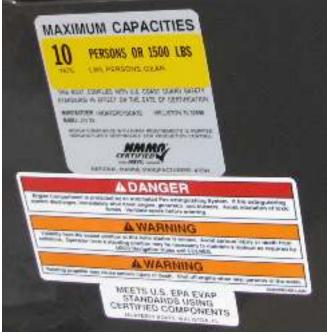
Typical Capacity Plate (Boats Up To 26 Feet) Note that the plate shown is for reference purposes only. Always refer to the capacity plate on your boat for actual maximum load capacities and persons.
