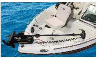
Typical Trolling Motor Mounted to Deck
