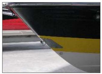
Typical Rope Locker Drain
