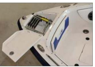
Typical Anchor/Rope Locker & Retractable Bow Boarding Ladder
