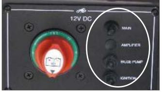
196MS Battery Switch Circuit Breaker Panel
