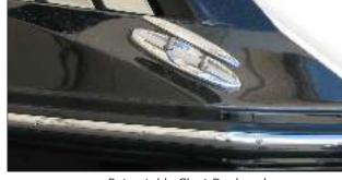
Retractable Cleat Deployed
