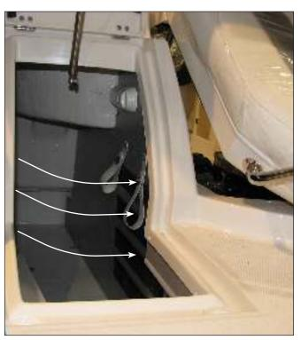
264FSC Engine Compartment Air Flow Through Storage Compartment
