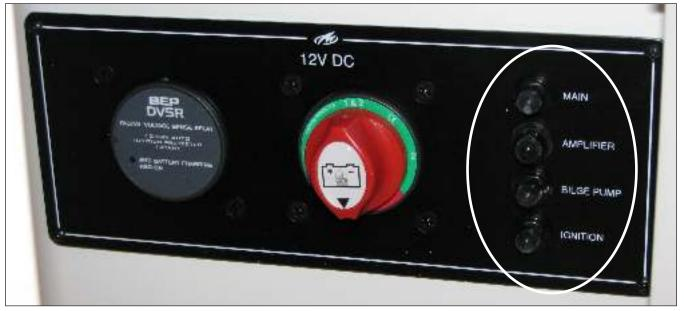
264FSC Battery Switch Circuit Breaker Panel
