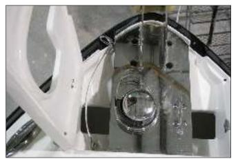
264FS/264FSX/264FSC Windlass, Chain Binder & Anchor Line Cleat
