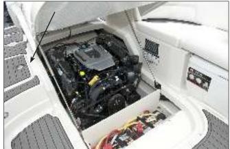
264FS/264FSX/264FSC Engine Compartment Access Hatch Open & Starboard Access Hatch
