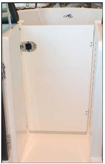
264FS/264FSX Walk-Thru Door Latched In The Closed Position
