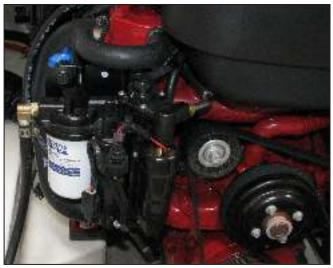
Typical Inboard Spin On Engine Fuel Filter
