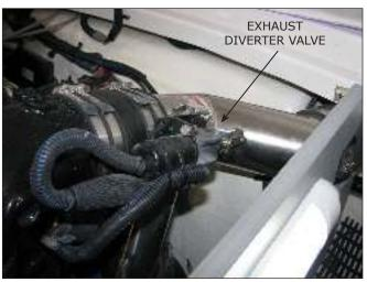
Exhaust System Diverter Valve
