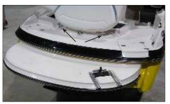
224FSC Engine Compartment Vents
