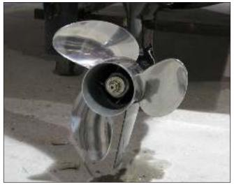
Typical Mercury Outboard Engine Propeller
