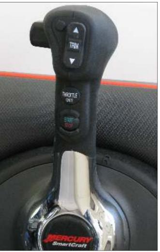
Mercruiser Single Engine Electronic Control Tilt/Trim Switch
