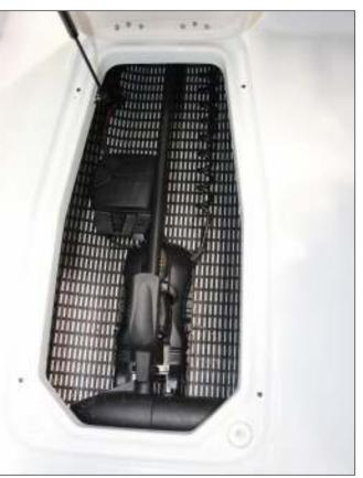
Trolling Motor Stowed in Center In-Floor Storage Compartment
