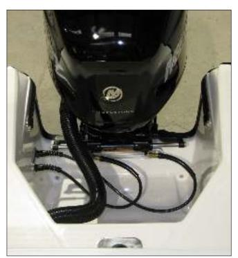
Mercury Outboard Engine Hydraulic Steering Cylinder
