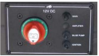
Typical Dual Battery Selector Switch Panel No Digital Voltage Sensitive Relay
