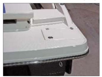
Typical Inboard Stern Ladder Compartment on Platform
