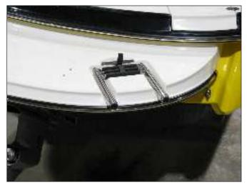
Typical Inboard Stern Ladder in Recess - No Hatch
