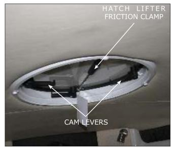
264FSC Deck Hatch Cam Levers & Hatch adjuster
