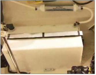
Typical Holding Tank & Charcoal Filter in Bilge
