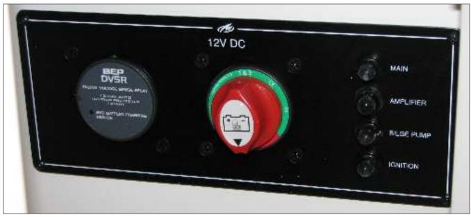
Typical Dual Battery Selector Switch Panel with DVSR
