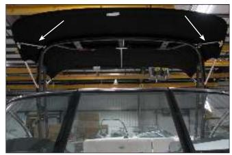
Open Front Top Section Supported With Stanchions on Each Side
