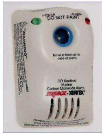
224FSC/264FSC Carbon Monoxide Detector
