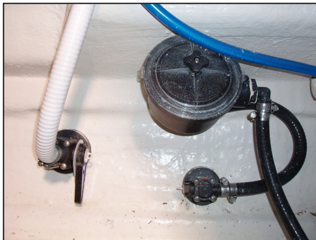
Holding Tank Overboard Discharge Thru-Hull Valve and Air Conditioner Sea Strainer
