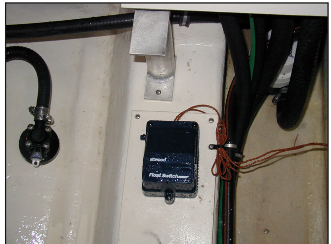
Automatic Float Switch for High Water Alarm and Emergency Bilge Pump Located Below the Engine Compartment Step.
